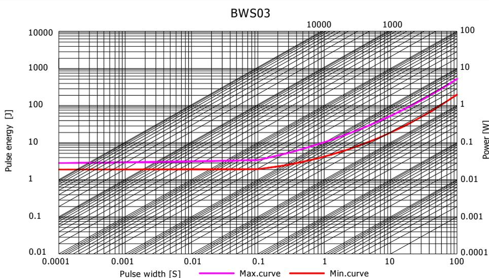
The max.curve is only valid for the resistance value 0.5m. The min.curve is only valid for the resistance value 4m. For other resistance values the area in between the max. and the min. curve is valid
