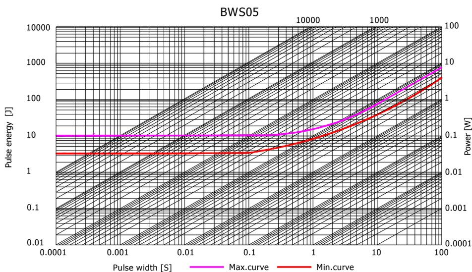
The max.curve is only valid for the resistance value 0.2m. The min.curve is only valid for the resistance value 2m. For other resistance values the area in between the max. and the min. curve is valid
